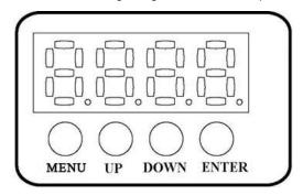
There are total 16 modes for control. When you press "MENU", the number will change gradually, from "A001" to "REST" in circle. Enter into the mode to adjust the effect you need.
